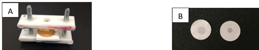
Figure 20. (A) A home-built blotting apparatus: four sheets of blot paper were layered on the Teflon base and the membrane was placed on top. A rubber O-ring (4-mm inner diameter) was placed between the membrane and top Teflon sheet. (B) the size comparison of two spots of aggregates obtained after filtration via the home-built blotting apparatus (left) and 48-well Bio Dot blotting apparatus (right). Each filter diameter is 13 nm.
